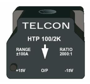
The HTP100/2K is a closed loop Hall Effect Current Transformer suitable for measuring currents up to 100A. The product provides an output current, galvanically isolated from the primary conductor into an external load resistance.
